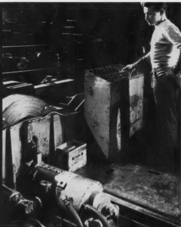
One man straps an average of 600 strip coils in 8 hours with this machine, which also tightens coils and squares up edges. Similar Signode machines have been in use since 1948.
